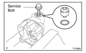
(b) Using a service bolt, pull it out together with the spring seat.
